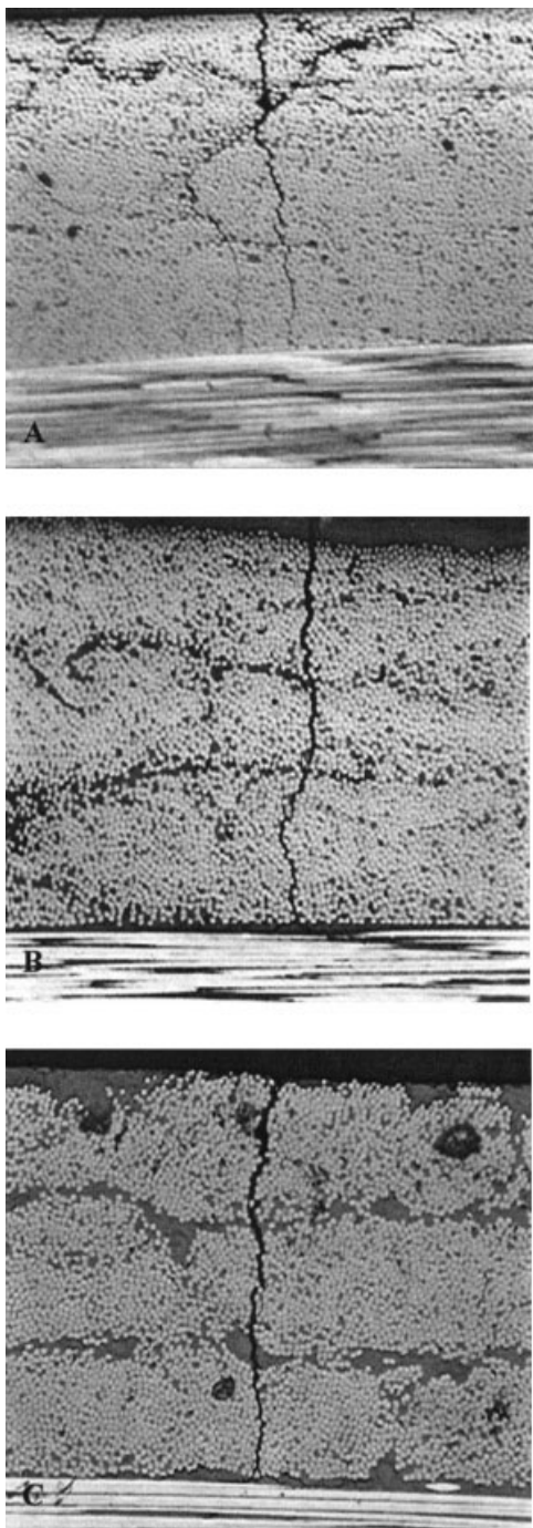
Figure 5 Reflected optical micrographs of cryogenically cycled laminates. (A) control, (B) DP 5031, (C) DP5045/Nipol 1472 ( \times 100 magnification).
